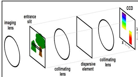
**Schematic of a spectral line camera.** The first lens images the scenery onto the entrance slit which selects a line from the image. Collimating lenses and a dispersive element spectrally separate the line, the result of which is recorded by a CCD. For our project we use the SpectroCam V10 spectral imagers supplied by SpectraPartners (400-1000 nm) combined with the WATEX 902h2 supreme low light monochrome camera (sensitivity 400 nm (50%) – 1000 nm (5%)).
