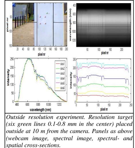
**Outside resolution experiment.** Resolution target (six green lines 0.1-0.8 mm in the center) placed outside at 10 m from the camera. Panels as above (webcam image, spectral image, spectral- and spatial cross-sections).
