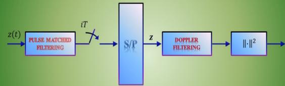
The design of **robust filters** for radar pulse-Doppler processing is considered.
