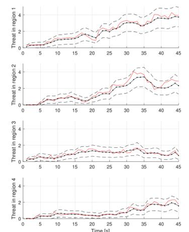
Fig. 2: Mean cumulative threat level and  $\pm 1$  standard deviation (square root of the variance, which is the sought after quality measure) in regions from 1 to 4. The ground truth value of the threat level is plotted with plain red line. The results are averages over 60 Monte Carlo runs.
