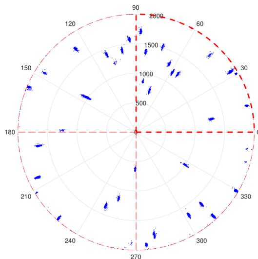
Fig. 1: Updated intensity  $\mu_k$  in an SMC-PHD filter. The particles (in blue) are projected on the subspace of position variables. Regions of interest are depicted with red dashed lines and numbered counter-clockwise with the first region plotted with a thicker line. The sensor with state  $x_o$  is located at the origin.
