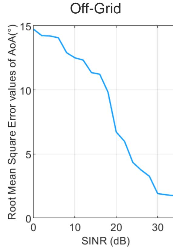
As expected in the off-grid case the RMSE converges to  $2^\circ$
