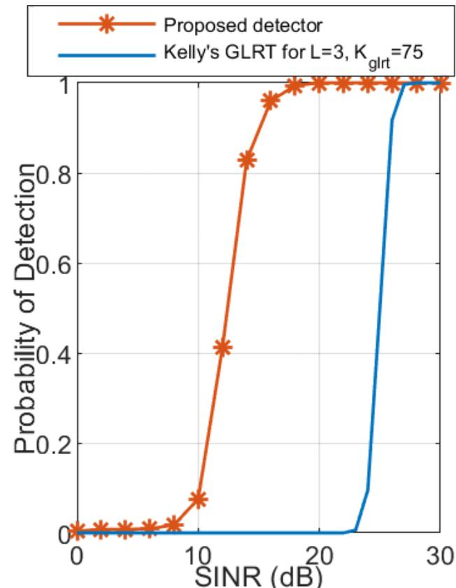
*Kelly's GLRT does not account for secondary data contamination caused by the redundant targets leads to the performance degradation of this classical detector.*
