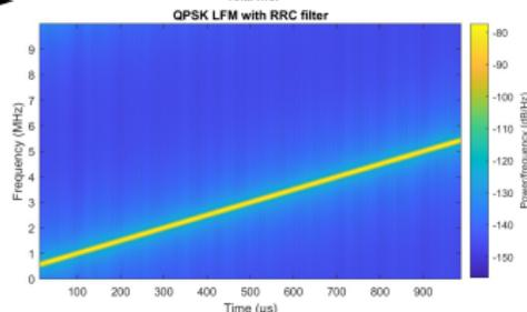
(d) QPSK-LFM waveform with Root-raised-cosine filter (Frequency Domain)
