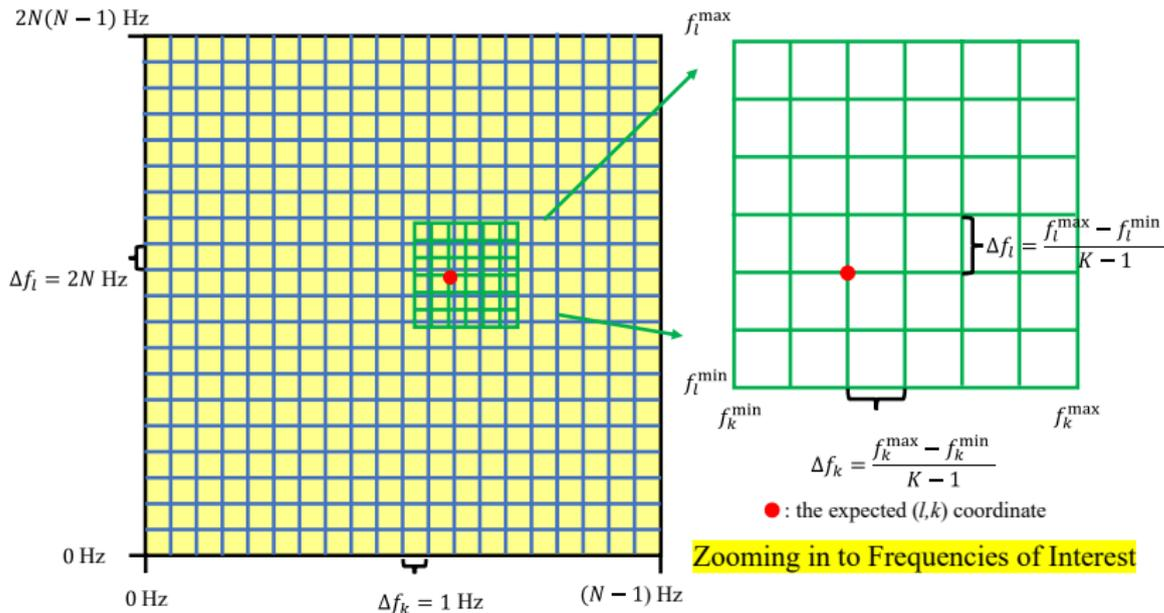
Figure: 2D Frequency Grid of DCFT (Left) and coherent-DCFT (Right).
