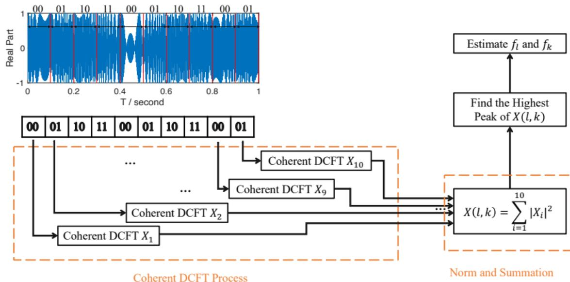
**Figure:** Example of non-coherent DCFT process when symbol length is **known** to be 10 symbols per chirp signal.
