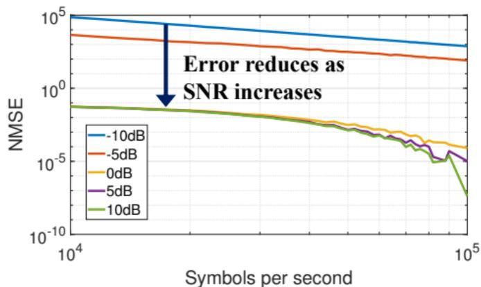
Figure: Performance of envelope method for the symbol rate estimation result.
