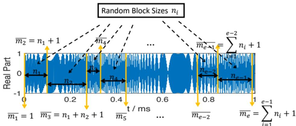
Figure: Diagram of random sampling method via different points  $\bar{m}_e$ .
